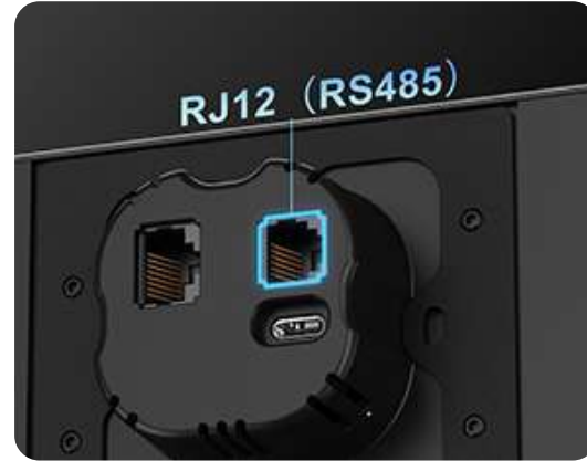
RJ12 Interface with RS485 Function
